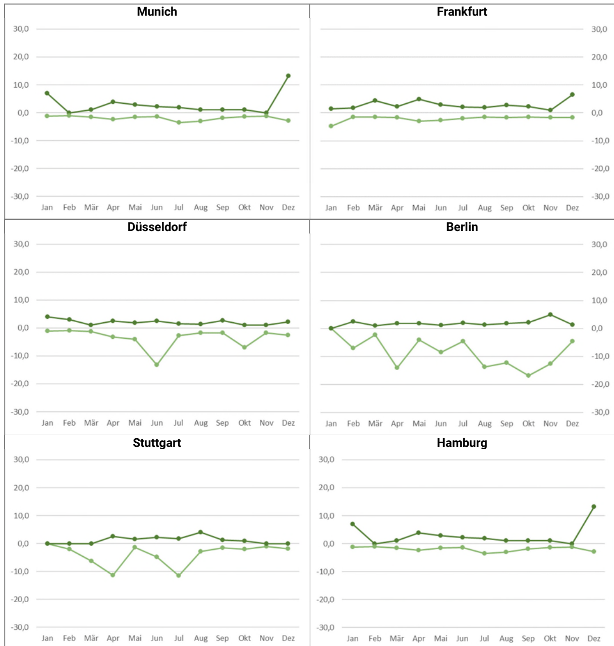
Fig. 2: Mean deviation in minutes of ATOT and STW for early (light green) and late (dark green) departures
