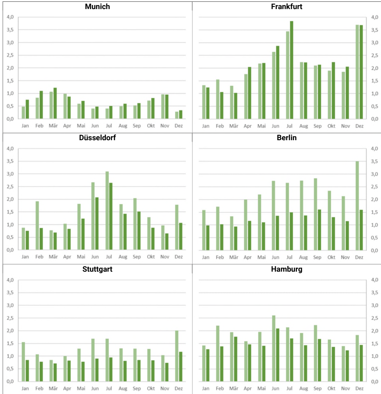
Fig. 13: Mean number of TSAT changes per regulated (light green) and non-regulated (dark green) flight and month without first TSAT, including deletions
