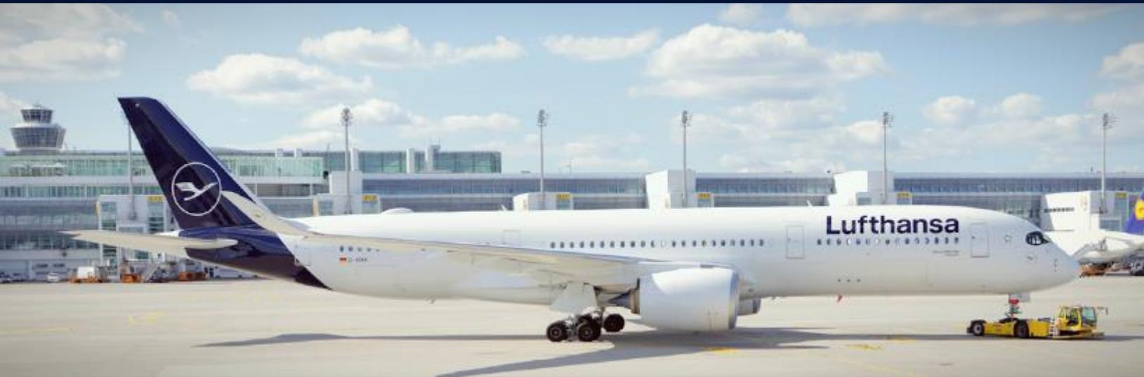
With our conventional and towbarless tractors we are able to move all aircraft currently approved for flight operations. By firmly clamping the front landing gear, the towbarless tractors can execute towing operations considerably faster than conventional towing tractors. In addition, towbarless tractors offer greater safety as the possibility of a broken towbar can be ruled out.
