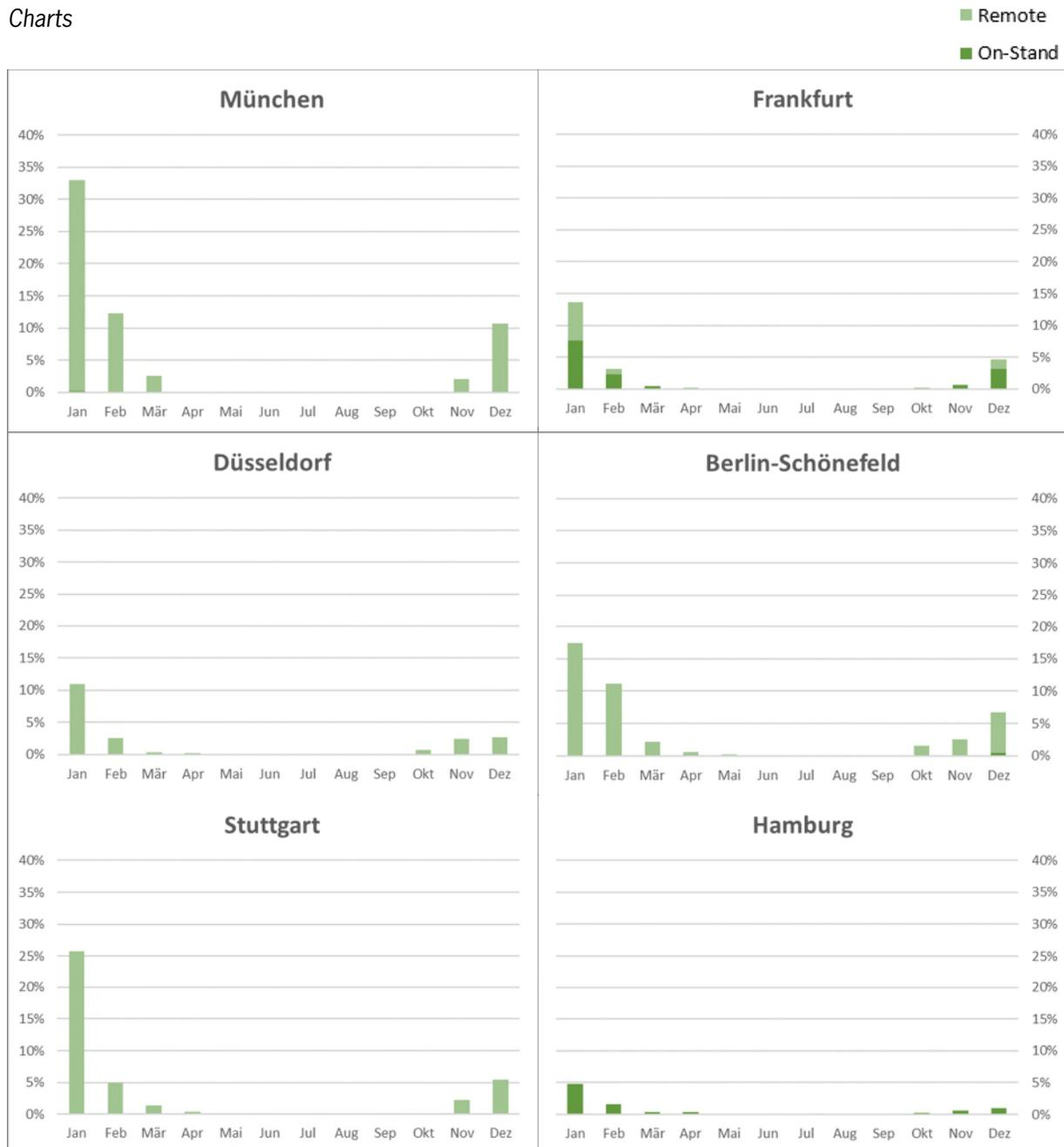
Fig. 4: Share of IFR departures 2019 requiring aircraft de-icing on stand (dark green) and remotely (light green)
