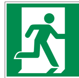
Escape route / emergency exit [right]
