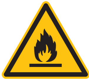
Warning, flammable materials
