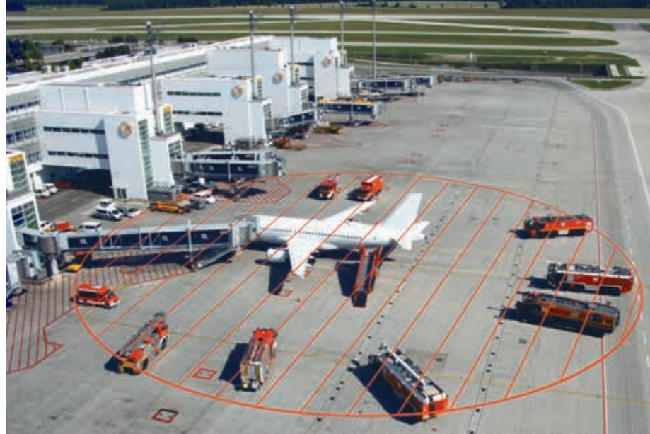
The stations set up during operations by the fire or emergency services may not be entered or driven through [red hatched area].
