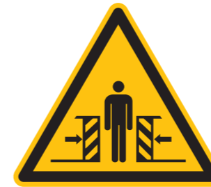
Warning, risk of crushing
