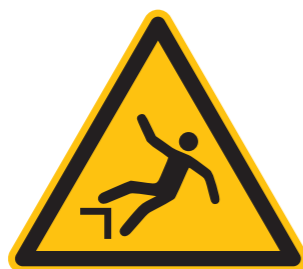
Warning, fall hazard
